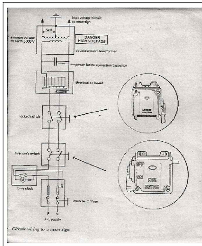
The voltages at which H V signs operate are between 600 V and 5000 V. Thus, a 10 kV display unit could be used provided its supply transformer is centre-tapped to earth.
