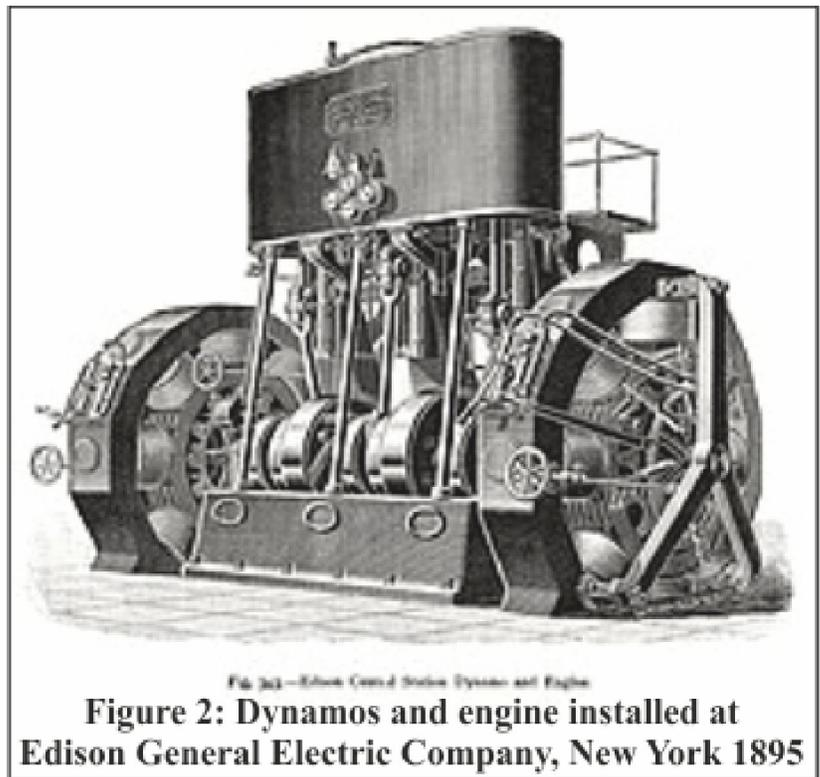
Figure 2: Dynamos and engine installed at Edison General Electric Company, New York 1895
