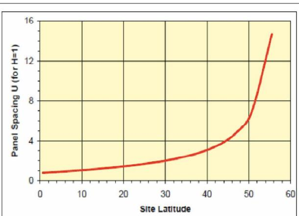
**Fig.3.5: Panel spacing versus Site Latitude**
