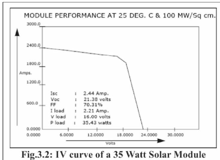
**Fig.3.2: IV curve of a 35 Watt Solar Module**
