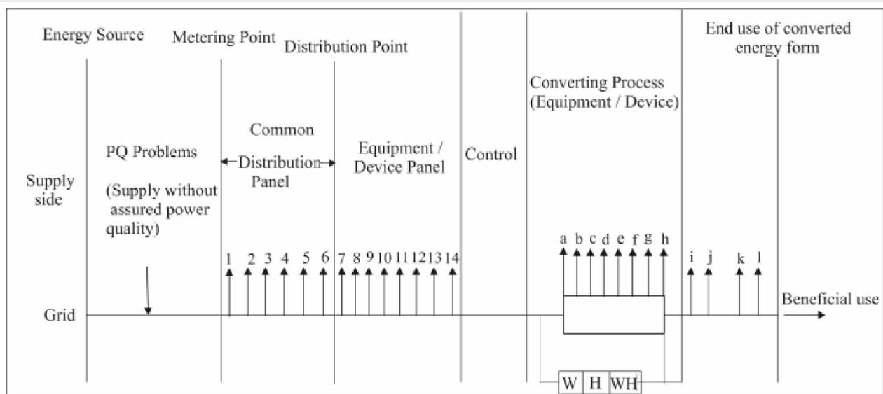
**Fig 8 Losses in power delivery circuit / process Legend**
