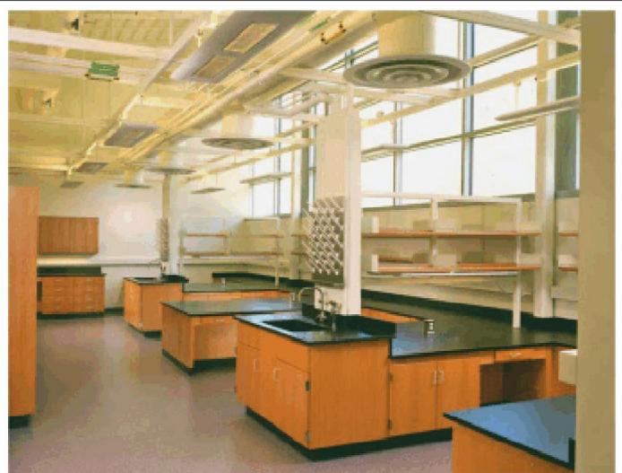
**Figure 11:** San Mateo County Forensic Laboratory incorporates integrated daylighting and lighting controls, contributing to anticipated energy consumption that is 50% less than mandated by California Title 24.
