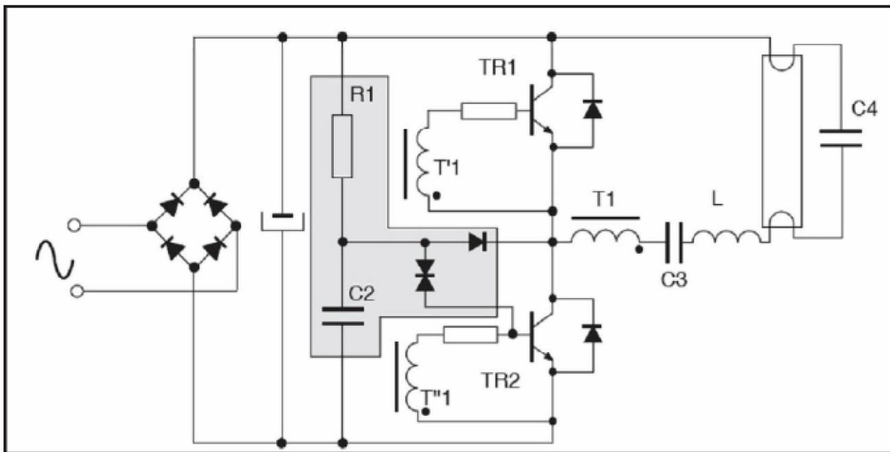
Electronic ballasts replace the starting and inductive elements of the conventional system. The aim of using an electronic ballast is to increase the operating mains frequency of 50 Hz to over 20 kHz.
